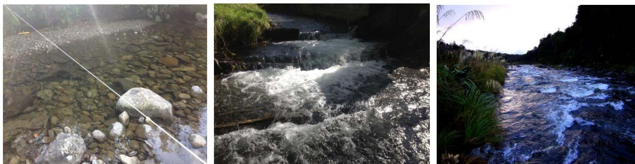
Figure 4: a) Gauging section with obstructions to flow, b) Highly turbulent flow not conducive to good gauging practice, c) Highly turbulent, high velocity, in-stream obstructions and fading light
