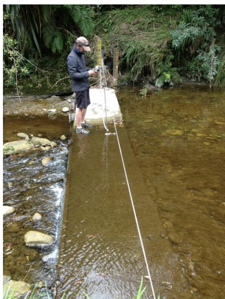
Figure 2a and b: a stable well-defined low-water control section, and b building an artificial low-water control / constriction for gauging low flows
